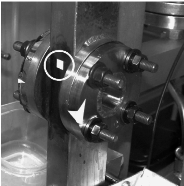
Fig. 6. IBBTL location monitored by LDV.
