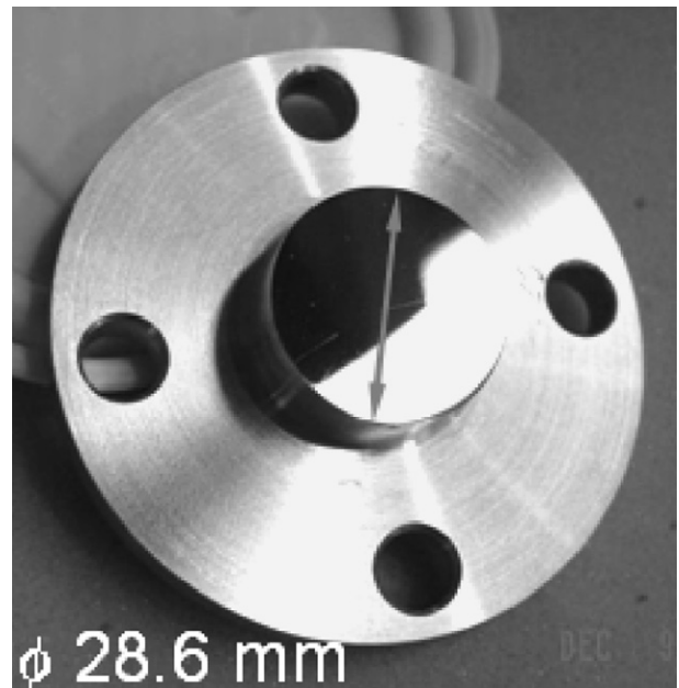
Fig. 3. Damage test specimen showing polished test surface.
